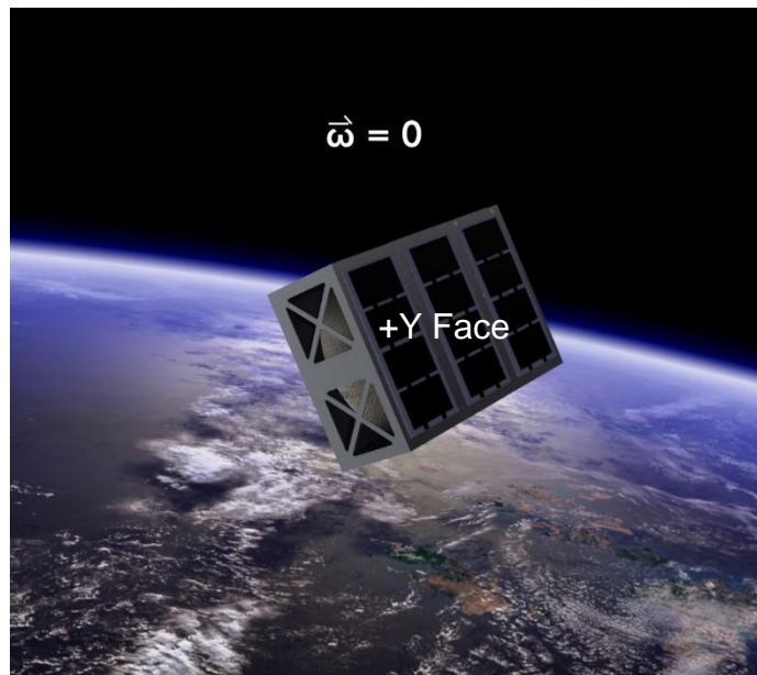
Figure 3: The spacecraft has successfully de-tumbled and is oriented in a thermal and power safe attitude. The +Y face is oriented towards the Sun.
